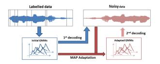
Figure 1: Overview of the MAP adaptation method for the GMM-based VAD.
